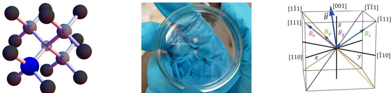
Fig. 1: Left , a schematic representation of the atomic structure of an NV center in a diamond crystal lattice, N - nitrogen atom, V - lattice vacancy, C - carbon atoms. Center , diamond samples used in laboratory research and prototype device development. Right , NV symmetry axes and laboratory-frame directions x , y , and z . A magnetic field B projects on to the four NV orientations, causing Zeeman shifts of the energy levels of the NV centers that can be measured using spectroscopic methods in combination with a laser and a microwave source [2].
